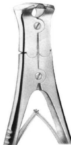
2419 Wire cutter. For ligature wires and pins. It is strong enough to bend archwire ends after distal cutting. Maximum cutting capacity: wires up to 1,5 mm. (.044"). With tunasten carbide insert.
